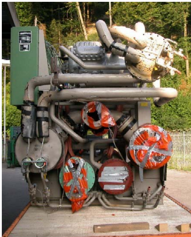
Fig. 4: Cleared refrigerating compressor at KKM
